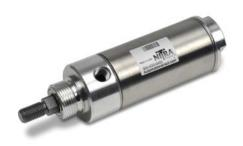
NITRA pneumatic stainless steel round body, interchangeable, non-repairable cylinder, 2 inch bore, 1/4 NPT ports, double acting, front nose mount.
