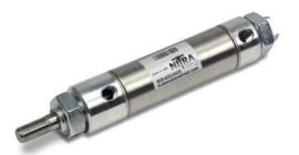
NITRA pneumatic stainless steel round body interchangeable, non-repairable cylinder, 1-1/4 inch bore, 1/8 NPT ports, double acting, double end mount, magnetic piston.
