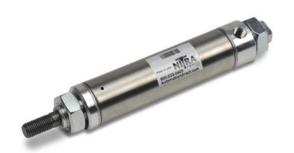
NITRA pneumatic stainless steel round body interchangeable, non-repairable cylinder, 1-1/4 inch bore, 1/8 NPT port, single acting, spring return, double end mount.
