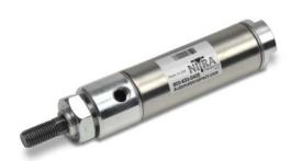
NITRA pneumatic stainless steel round body interchangeable, non-repairable cylinder, 1-1/4 inch bore, 1/8 NPT ports, double acting, front nose mount.
