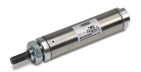
NITRA pneumatic stainless steel round body interchangeable, non-repairable cylinder, 1-1/4 inch bore, 1/8 NPT port, single acting, spring return, front nose mount.
