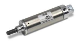
NITRA pneumatic stainless steel round body, interchangeable, non-repairable cylinder, 1-1/2 inch bore, 1/8 NPT port, single acting, spring return, rear pivot mount (pivot pin included). Cylinder cannot be double end mounted.
