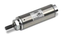
NITRA pneumatic stainless steel round body, interchangeable, non-repairable cylinder, 1-1/2 inch bore, 1/8 NPT port, single acting, spring return, front nose mount.
