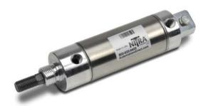
NITRA pneumatic stainless steel round body, interchangeable, non-repairable cylinder, 1-1/2 inch bore, 1/8 NPT ports, double acting, rear pivot mount (pivot pin included). Cylinder cannot be double end mounted.
