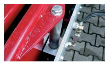
This saw mill uses a DryLin® linear bearing with iglide® J plastic liner for the angle stops.
