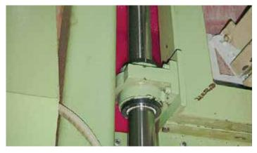
This heavy duty application has run reliably for more than three years thanks to DryLin® RJUM-01 linear bearings
