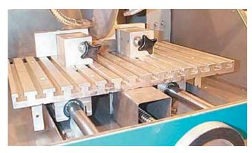
DryLin® R linear plain bearings on supported aluminum shafts are used in the guide for this cutting table. The DryLin® components stand up to the high levels of dust and dirt, and offer accurate, smooth operation.
