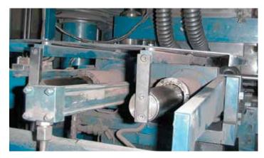
Despite the high stresses from abrasive particles and powder particles, this compactor unit can extend maintenance-free uptime by up to two years after switching to DryLin® R linear bearings.
