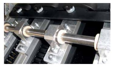
To enable fast, and precise adjustment of a production line without the need for downtime, DryLin® precision linear guides were utilized.
