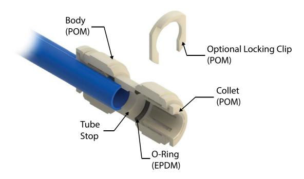
Push-to-Connect Fitting Cut-away Diagram
