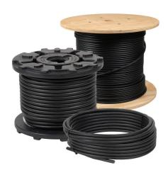
Helukabel Traycontrol® 600V from AutomationDirect is available in sizes from 20AWG to 4AWG with 2 to 41 unshielded conductors. Individual conductors are bare copper and stranded for flexibility, with black PVC/Nylon insulation and marked with numbers for easy identification. A convenient insulated ground conductor, green with a yellow stripe, is included in the conductor count of each cable with conductor counts higher than two.
