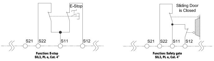
\* To achieve the safety classification, cross fault wiring must be installed.
