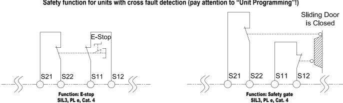
Safety function for units with cross fault detection (pay attention to "Unit Programming"!)
