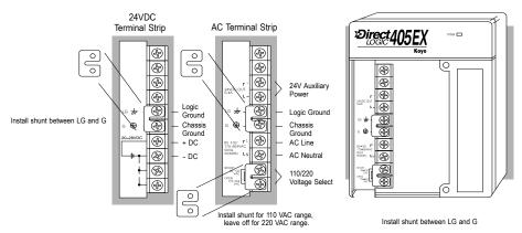
Recommended screw torque: 10.6 lb-in (1.2 Nm)
