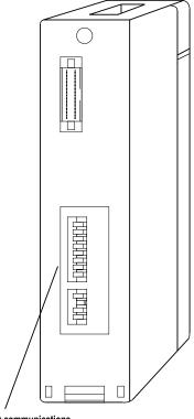
DIP Switches for communications and Protocol Setup
