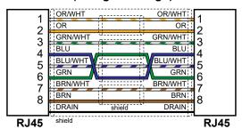
12345678 8-pin RJ45 Connector (8P8C)
