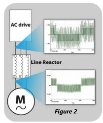
placed at the output of the drive, can help reduce the voltage spikes going from the drive to the motor. Line reactors are used in many instances when the motor is located far from the drive [see Figure 2].
