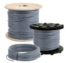
Control and signal cable from Quabbin is available in sizes from 24 AWG to 16 AWG with up to 25 conductors. These are available either in unshielded or shielded constructions. Individual conductors are stranded tinned copper with color coded insulation for easy identification, with an industry standard PVC chrome gray jacket. Shielded versions include an overall aluminum mylar foil tape with a tinned copper drain wire for maximum effectiveness against external electrical noise interference.
