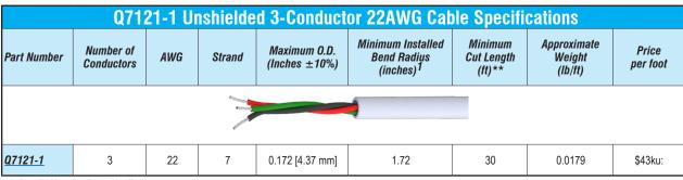
1. Installed bend radius ≥ 10x diameter
