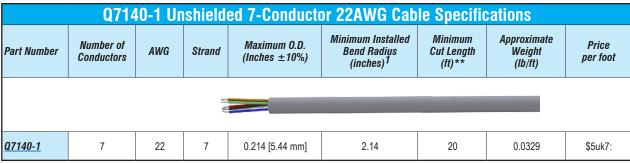
1. Installed bend radius  $\geq$  10x diameter
