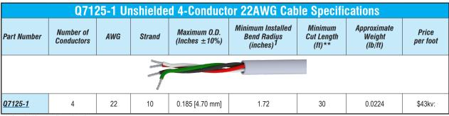
1. Installed bend radius ≥ 10x diameter
