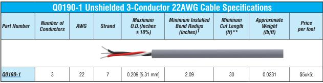
1. Installed bend radius ≥ 10x diameter
