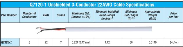
1. Installed bend radius ≥ 10x diameter
