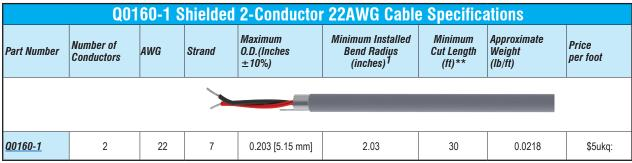
1. Installed bend radius ≥ 10x diameter
