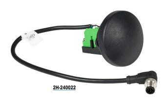
The IDEM Mechanical Pushbutton is a mechanically activated pushbutton with 1 NO and 1 NC set of contacts. This pushbutton was designed for use with any two-hand control system. This pushbutton is supplied with a 250mm [9.84 in] flying lead with a 5-pin M12 male plug. The plug makes it easy to connect to the PCB connection board which is part of IDEM's two-hand control stations.
