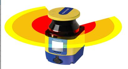
Datalogic Safety Laser Scanners can manage two simultaneous warning zones and one safe zone. Safe zones can extend up to 5.5 m [18.04 ft], depending on the model, over an angle of 275 degrees. Warning zones can extend 40m [131.2 ft].
