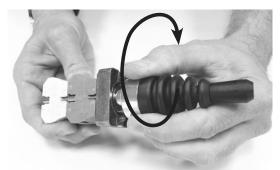
Twist clockwise until it clicks into place. Carefully tighten the securing screws. Do not over-tighten. (4.5 lb·in) If the operator is not "clicked" into position before the screws are tightened, the switch will not work properly.
