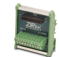
ZL-RTB20 20-pin feed-through connector module
