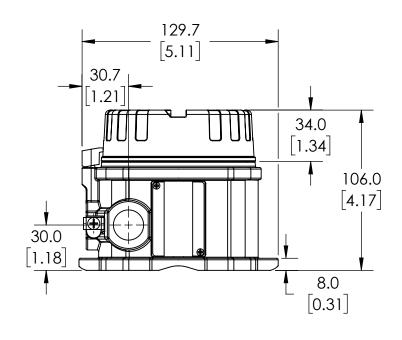
E+H ITEMP PROGRAMMABLE TEMPERATURE TRANSMITTER TMT142B-1E60 1W9 AutomationDirect.com 1-800-633-0405
