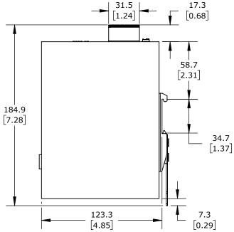
WAGO INDUSTRIAL LEAN MANAGED ETHERNET SWITCH, 8 PORTS, (8) POE+ 10/100/1000BASE-T (RJ45) AND (2) SFP COMBO GIGABIT PORT(s), MODBUS TCP AND SNMP, -40 TO +60 DEG C, METAL HOUSING, IP30, 35mm DIN RAIL MOUNT
