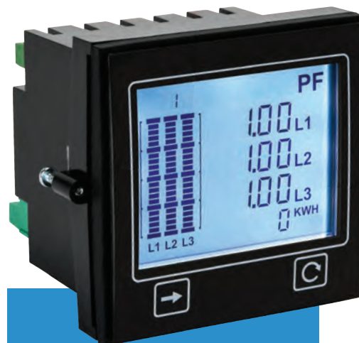
Figure 2: In addition to basics like current and voltage monitoring, the Trumeter ADM100W-HPS graphical power meter includes advanced functions like power factor, THD, and energy monitoring. Modbus connectivity provides expanded reading of data values, like phase angle or alarm(s).
