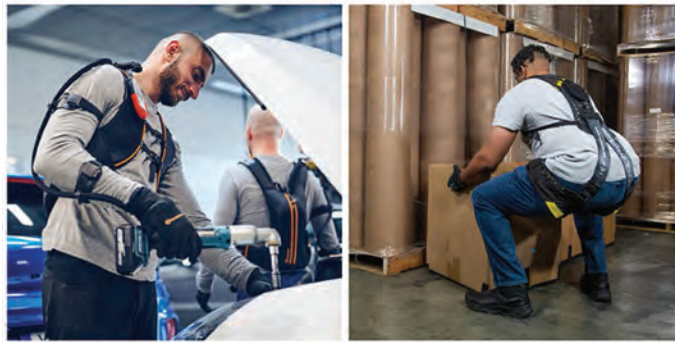
● Figure 2: Active soft hand exoskeleton relieves strain for worker using heavy hand tools (left). Passive back exoskeleton (right) consists of straps and elastic bands that provide back support for workers lifting heavy objects or bending over for large amounts of time (right). (Source: Wikipedia)
