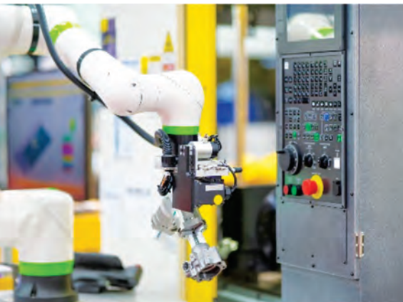
Figure 3: Classic industrial robots are kept in cages to protect workers from high velocity movements (left). Robots are designed for human interaction, with rounded edges and low-speed, low-force motion (right).
