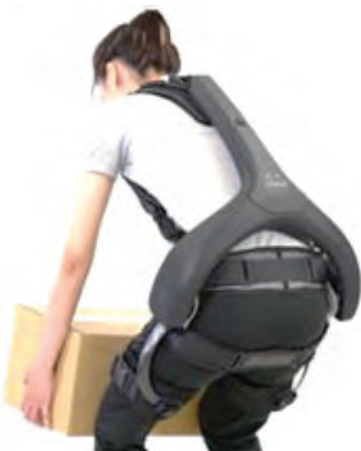
Figure 1: This type of rigid exoskeleton for powered lifting support assists the wearer in moving heavy loads, reducing risk of back strain. (Source: Wikipedia)
