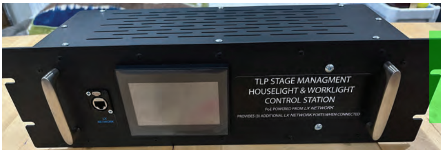
Figure 3: The stage manager’s lighting and sound controls are based on a user-friendly AutomationDirect C-more HMI, which is rack-mounted into a portable arrangement for convenient use wherever it is needed.
