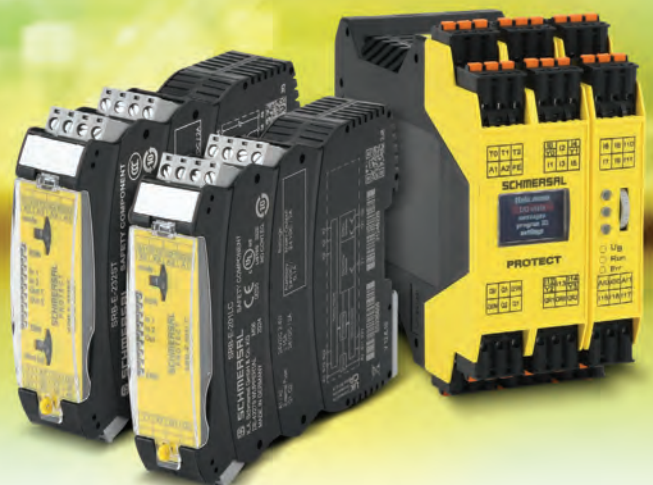
Figure 4: Configurable safety relays in the Schmersal PROTECT SRB-E product line can handle as many as 10 safety inputs and 5 safety outputs, as well as supporting many different applications. Each is compatible with monitoring all conventional safety devices.
