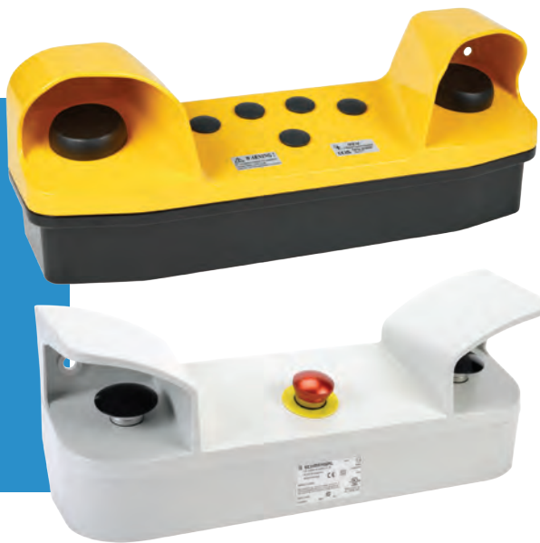
Figure 3: Two-hand safety control panels like these from IDEM (top) and Schmersal (bottom) feature guard hoods over the actuators to prevent operators from running the equipment with only one hand or from the back side of the panel.
