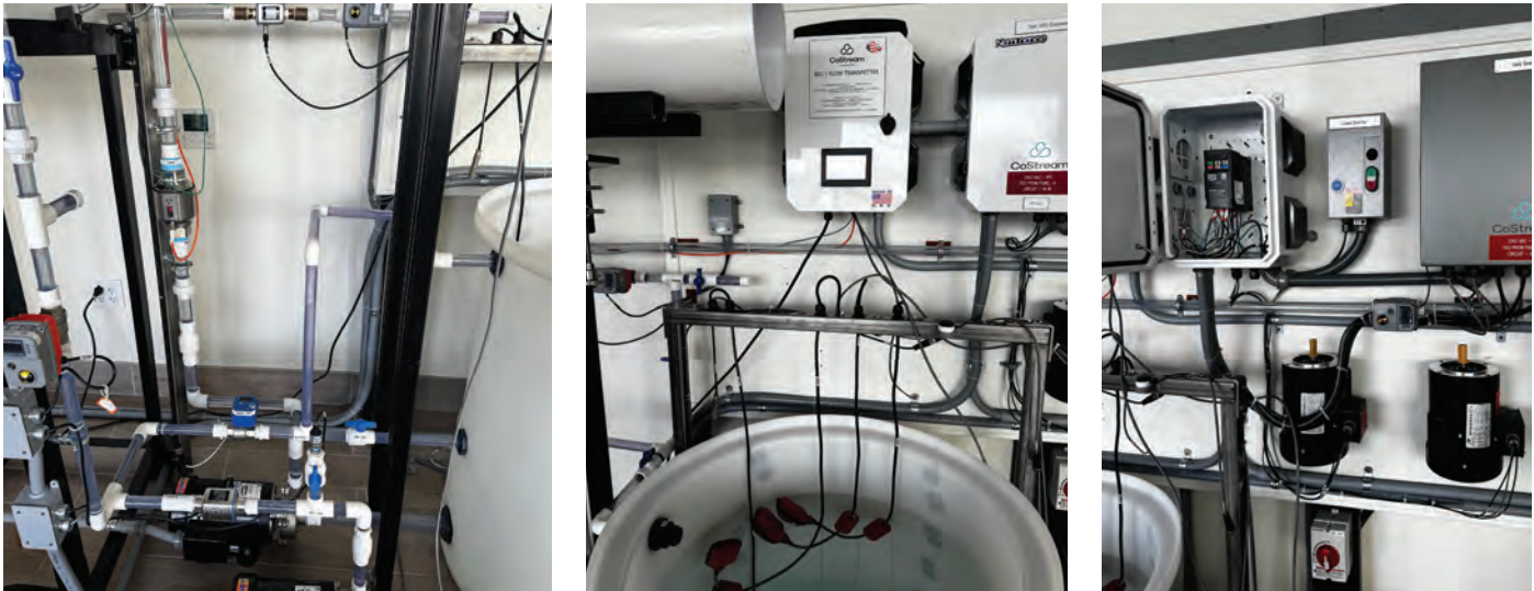
● Figure 2: The test lab brings together hardware a typical small utility would encounter: (a) A flow transmitter with transparent piping that lets students see water flow in real time, (b) A tank with float sensors, and (c) motors with their wiring routed for easy access with a clamp meter and a VFD to run them.
