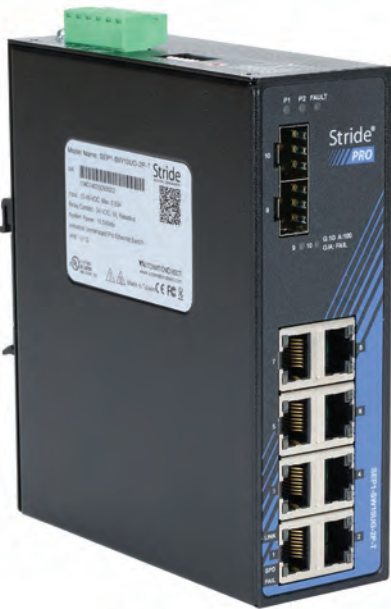
● Figure 1: AutomationDirect's STRIDE PRO Unmanaged+ Gigabit switches provide high-functionality features like IGMP snooping and VLAN support for network segmentation. It can be easily configured via DIP switch.
