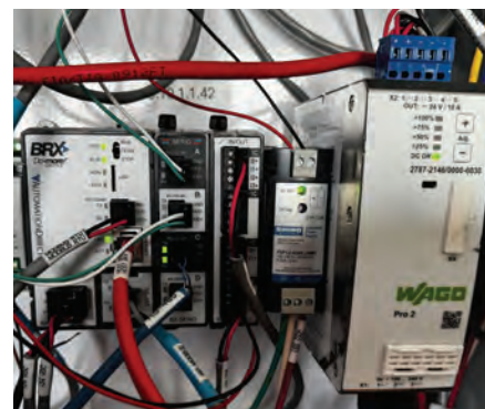
● Figure 3: PLC enclosures include equipment such as switches, breakers, power supplies, the PLC, and even a motion sensor for simulating panel intrusion alarms. The wiring in the test lab BRX PLC cabinet is slightly messy by design to make troubleshooting as realistic as possible.
