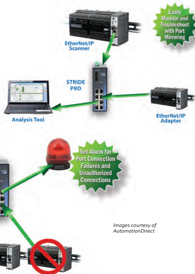
Figure 3: AutomationDirect Stride PRO industrial unmanaged+ Ethernet switches incorporate IT tools like IGMP snooping and port mirroring, along with more OT-focused options such as port disconnect alarms.
