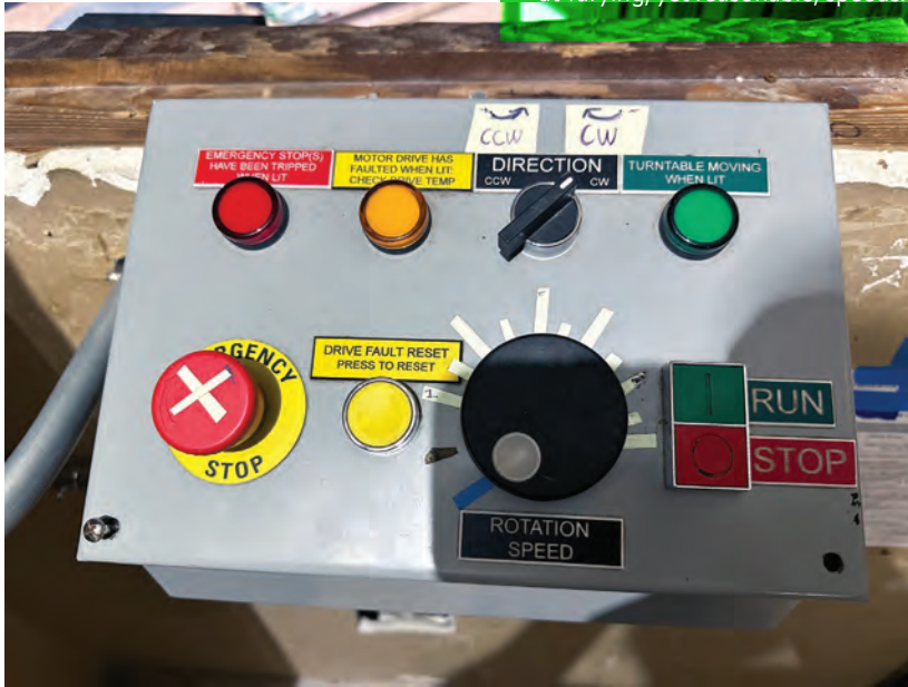
Figure 3: The operator console shown here uses several buttons, lights, and an e-stop button sourced from AutomationDirect to provide a simple way for stagehands to operate the stage revolve forward and backward at varying, yet reasonable, speeds.
