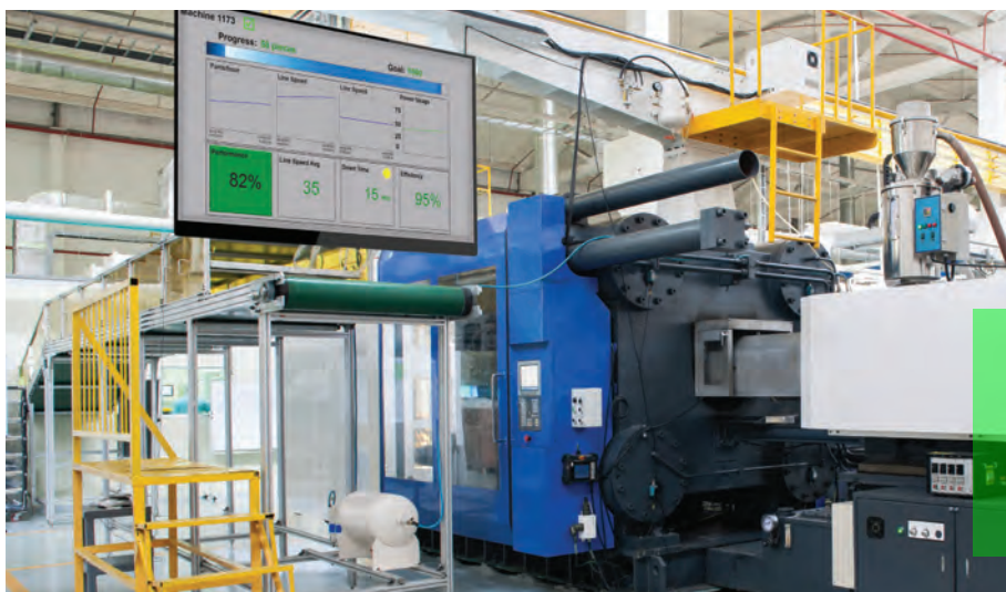
Figure 2: Powered by a headless HMI, large format displays can provide key process information, keeping plant staff informed even at a distance.
