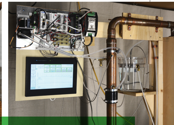
(RIGHT) Figure 2: The dephlegmator is at the top of a packed column (between the black sleeve and tri-clamp fitting) to create reflux. Water flow and the resulting cooling must be controlled by the PLC to maintain the ideal alcohol content setpoint.
