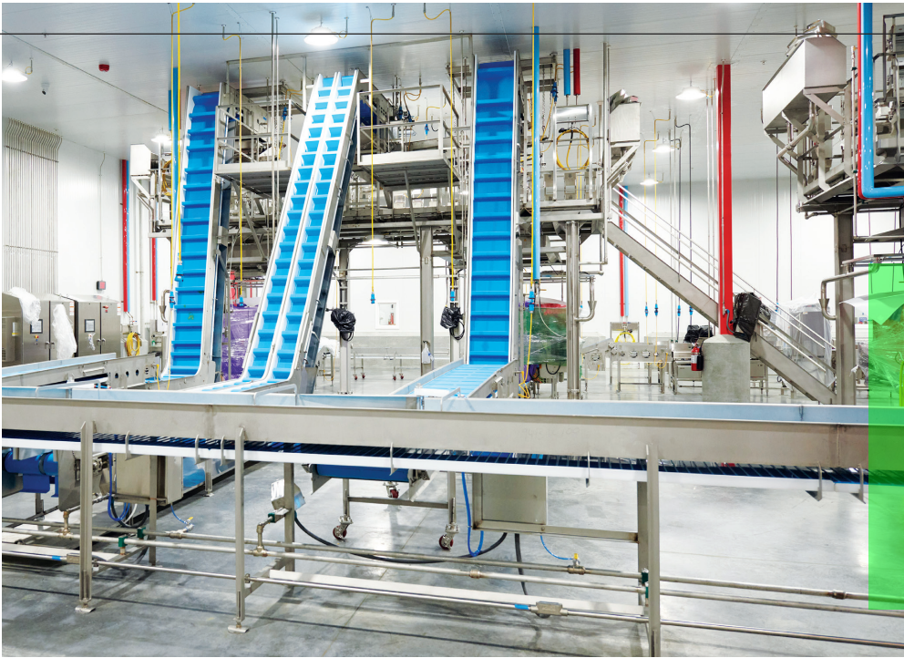
Figure 1: A turnkey automation solution in the food processing industry includes sophisticated controls and sanitary, washdown-resistant designs for cooking equipment, product conveyors and associated utilities such as air exhaust and wet well systems.
