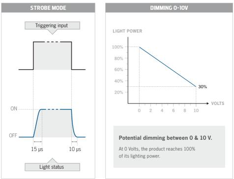
The product is optimised for a lifespan >50kh in a 40°C atmosphere. In strobe mode, the strobing time is directly equivalent to the time during which the strobe entry is activated.
