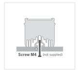
You can also use M4 screws (not supplied) fastened directly into Aluminium profile with a tightening torque from 0.5 to 1.5 Nm. We also recommend the use of a thread-locker (not supplied) to avoid any risk of loosening.
