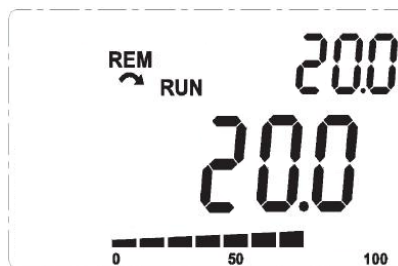
Figure 16.3: Example of HMI in the monitoring mode to use the PID controller
