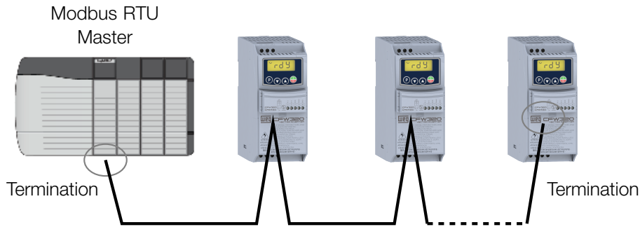
Figure 3.1: Modbus RTU network installation example
