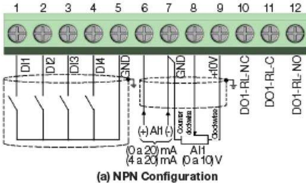
**For a potentiometer**, the outside wires go to terminals 7 and 9, and the center wire, the wiper, goes to terminal 8.
