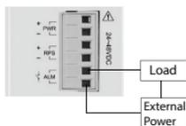
The 852-1812/010-000 has one set of relay alarm output. This relay contact uses two contacts of the terminal block on the 852-1812/010-000 top panel.
