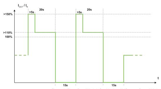
Figure 43: "Power Boost" Mode in Combination with "Constant Current" Mode
