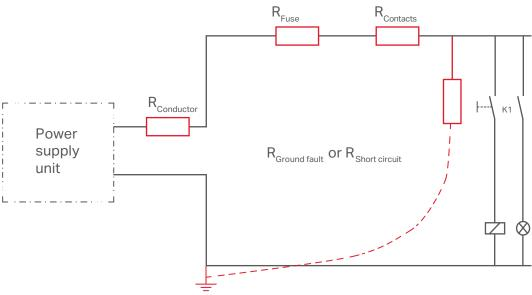
Figure 44: Loop Impedance
