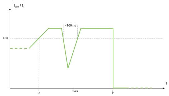
Figure 42: "Electronic Circuit Breaker" Mode
