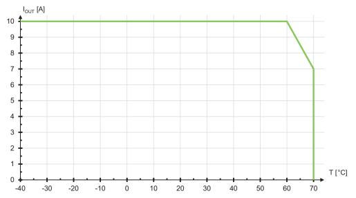
Figure 37: Derating (Temperature-Dependent)
