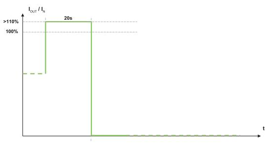
Figure 40: "Constant Current with Latching Shutdown" Mode
