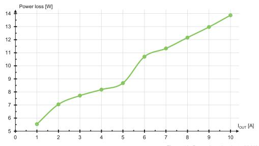
Figure 12: Power loss (typ.) at 400 VAC
