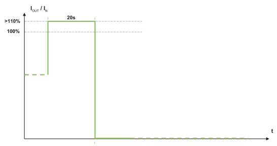
Figure 40: "Constant Current with Latching Shutdown" Mode
