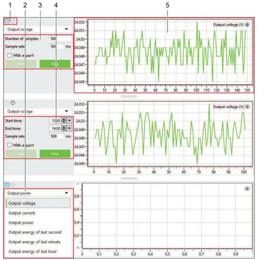
Figure 34: Display Section: "Measurement Recording"
