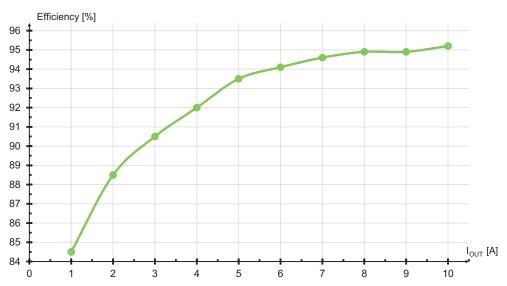
Figure 11: Efficiency (typ.) at 230 VAC
