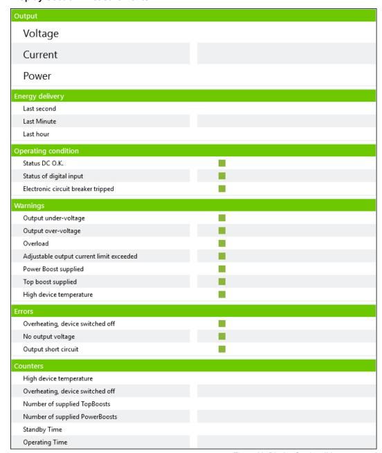
Figure 33: Display Section: "Measurements"
