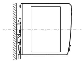
Figure 14: Position of the DIN-35 rail
