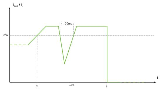
Figure 42: "Electronic Circuit Breaker" Mode
