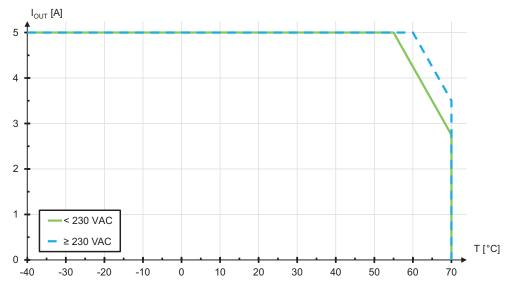
Figure 37: Derating (Temperature-Dependent)
