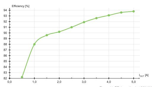
Figure 11: Efficiency (typ.) at 230 VAC
