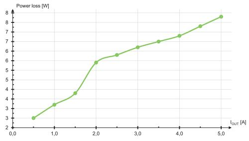
Figure 12: Power loss (typ.) at 230 VAC
