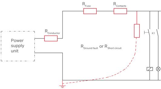
Figure 44: Loop Impedance
