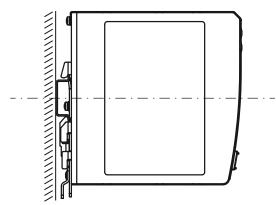
Figure 14: Position of the DIN-35 rail
