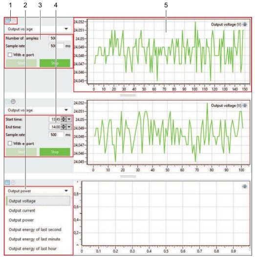
Figure 34: Display Section: "Measurement Recording"
