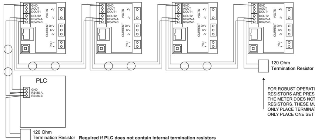
FOR ROBUST OPERATION, ENSURE MODBUS BIASING RESISTORS AND TERMINATION RESISTORS ARE PRESENT ON THE BUS. THE METER DOES NOT CONTAIN INTERNAL BIASING RESISTORS OR TERMINATION RESISTORS. THESE MUST BE FITTED EXTERNALLY. ONLY PLACE TERMINATION RESISTORS AT ENDS OF TWISTED-PAIR TRUNK CABLE. ONLY PLACE ONE SET OF BIASING RESISTORS ON THE BUS
