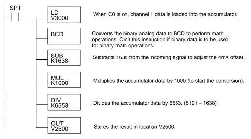
Example 2: Scaling Unipolar and Bipolar Input Signals Here's how you would write the program to perform the engineering unit conversion for a 0–5V, 0–10V,  $\pm 5$ ,  $\pm 10$ , 0–20mA or  $\pm 20$ mA input signal. The example assumes the analog data is in V3000.
