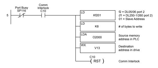
The DL06/260 CPUs support the Modbus Read (MRX) and Modbus Write (MWX) instructions. These instructions allow you to enter Modbus Slave Memory Addresses (no need to use octal addressing conversions to communicate with the drive).
