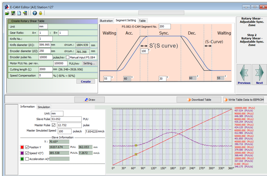
Figure 7-106 SureServo2 Pro setting interface for [Rotary Shear - Adjustable Sync. Zone]
