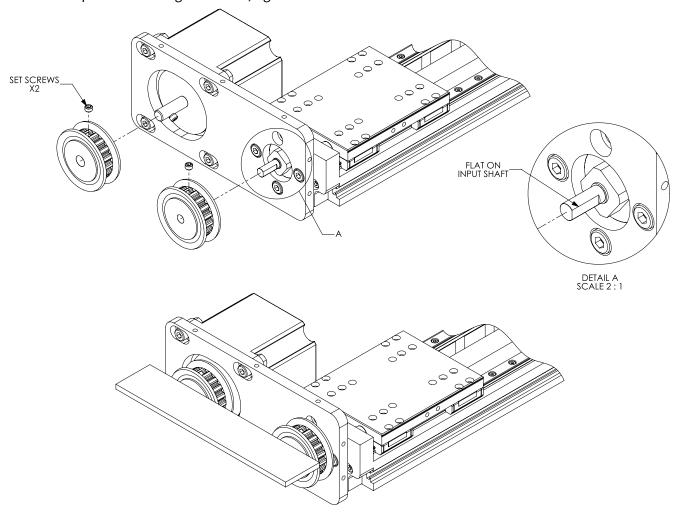
5) Attach the belt to the pulleys. If needed, loosen the bolts on the motor, adjust the motor position to change the tension on the belt, and re-tighten the bolts.
