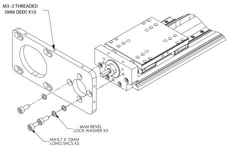
2) Secure the NEMA 23 stepper motor to the mount using the four (4) supplied bolts and washers.
