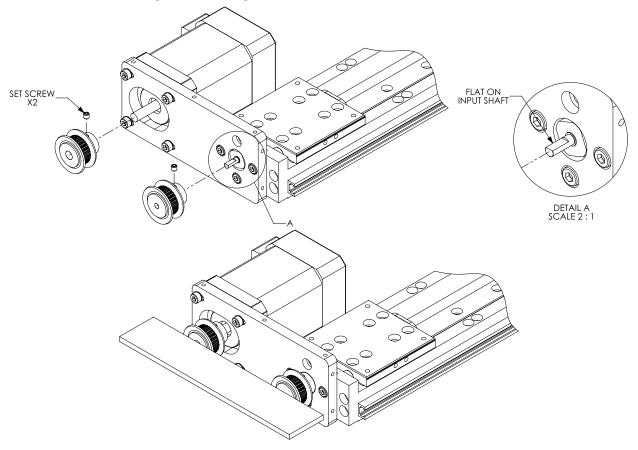
5) Attach the belt to the pulleys. If needed, loosen the bolts on the motor, adjust the motor position to change the tension on the belt, and re-tighten the bolts.
