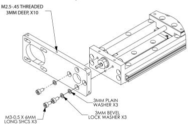
2) Secure the NEMA 14 stepper motor to the mount using the four (4) supplied bolts and washers.
