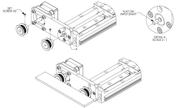
5) Attach the belt to the pulleys. If needed, loosen the bolts on the motor, adjust the motor position to change the tension on the belt, and re-tighten the bolts.
