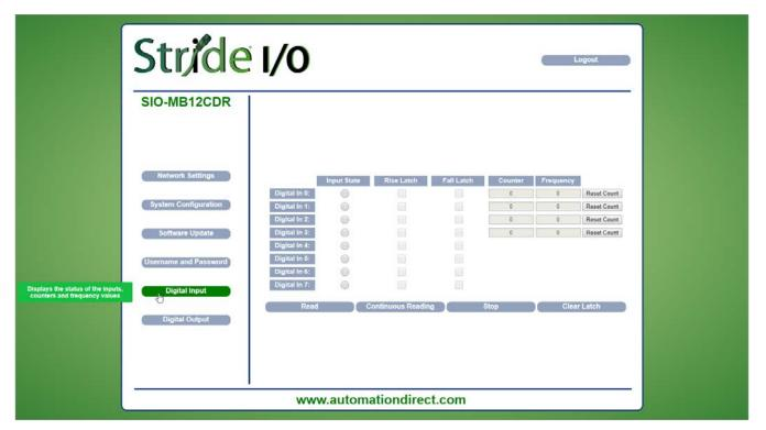
This page displays the state of the digital inputs and their associated latches.
