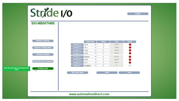
This page displays the values of the analog inputs in the unit of measurement defined by the "Input Type". Each input is electrically isolated from all others and can be configured independently.
