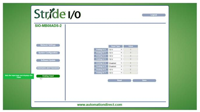
This page displays the values of the analog inputs in the unit of measurement defined by the "Input Type". Each Input can be disabled selecting "Disabled" in the combobox under the column "Input Type".
