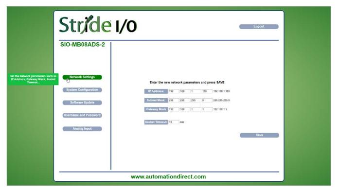
On the Network Settings page, set the Ethernet communication parameters.
