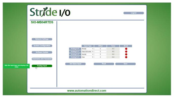
This page displays the values of the analog inputs in the unit of measurement defined by the "Input Type". Each input is electrically isolated from all others and can be configured independently.
