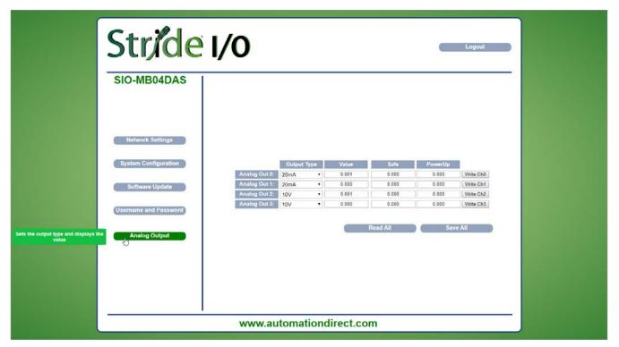
This page displays the values of and allows writing to the analog outputs in the unit of measurement defined by the "Output Type". Each Output can be configured independently as voltage or current. Each output is electrically isolated from all others.
