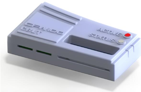
**02** - Green LED (STATUS): indicates the serial communication service of the CFW100-CBLT module is active.
