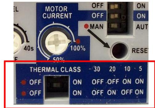
Figure 7 – Thermal Class Dip Switch Location
