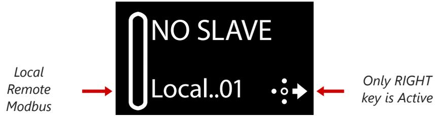
By pressing the Right key, the user will be taken directly to the Modbus address selection menu:
